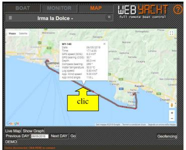
By clicking on "Geofencing" you can draw areas on the map and receive alarm SMS if the boat enters or leaves the perimeter
