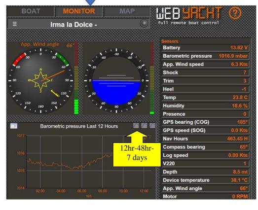
On the Monitor panel: on the right, Sensors represents all instrument values in real time. By clicking on any one, the graph for that value appears on the left. In the graph there are buttons to see the last 12 hours, 2 days or 7 days (click on the top right of the graph to change).
